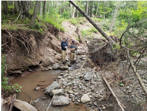
Figure 1 Mark Tollefson (UCSWCD) surveying with Nate Parker (SUNY Ulster Student, Watershed Conservation Corps) at a future stream restoration site on the Panther Kill in Shandaken, NY. The team is monitoring geomorphic and habitat conditions prior to stream restoration. The restoration work will address geomorphic instability and erosion into fine sediment sources causing water quality impairment.
